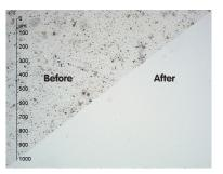
Oil cleanliness maintained at better than new levels (Down to 13/11/8 (ISO 4406: 1999) - Class 2 (NAS 1638).
